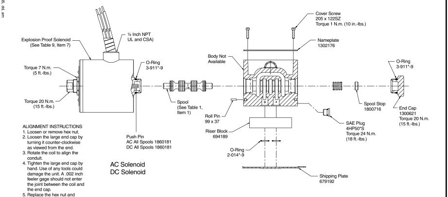
D3W Single AC Solenoid Model D3W Single DC Solenoid Model
