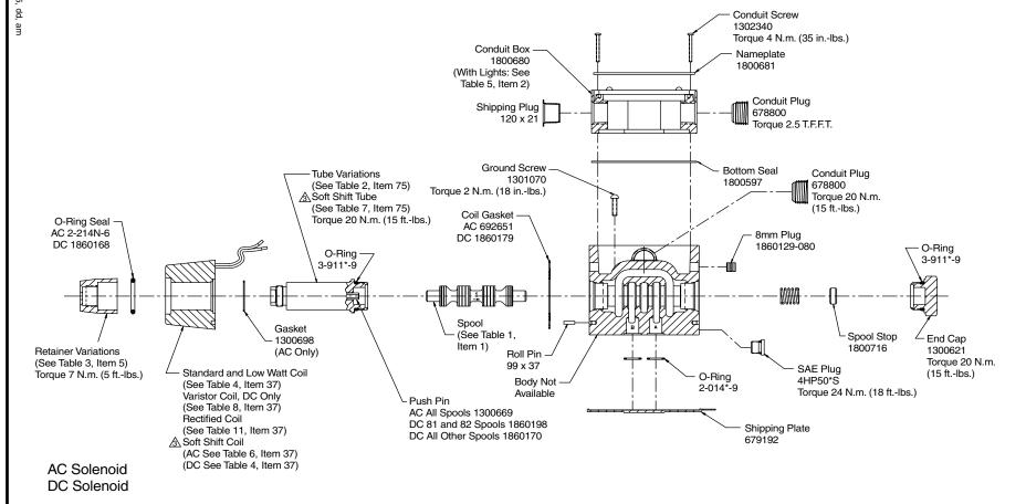
D3W Single AC Solenoid Model D3W Single DC Solenoid Model
