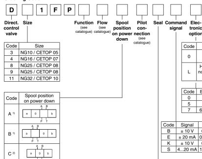
Standard for 0 spool B, E, R Hybrid valve 24V normaly closed for L spool code Z Code Electronic option 6 + PE 0
