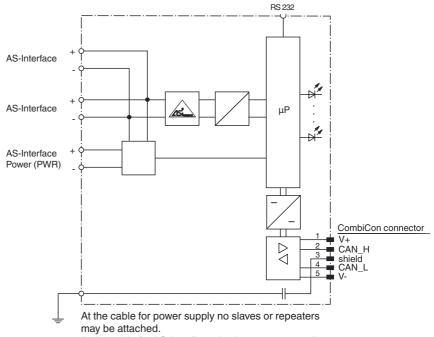
At the cable for AS-Interface circuit no power supplies or further masters may be attached.
