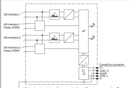
AS-Interface circuit 1 and 2 are supplied from different power supplies. The gateway is supplied from circuit 1. At the cable for power supply no slaves or repeaters may be attached.
