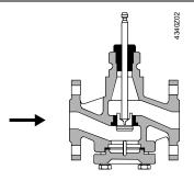
For all nominal sizes, a guided slot plug is used that is directly connected to the valve stem.
