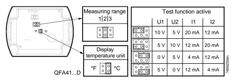
The setting elements are located inside the cover. A setting element consists of 6 pins and a jumper. It is used for selecting the required temperature measuring range and for activating the test function. Types with LCD display have a second setting element with 4 pins and a jumper.
