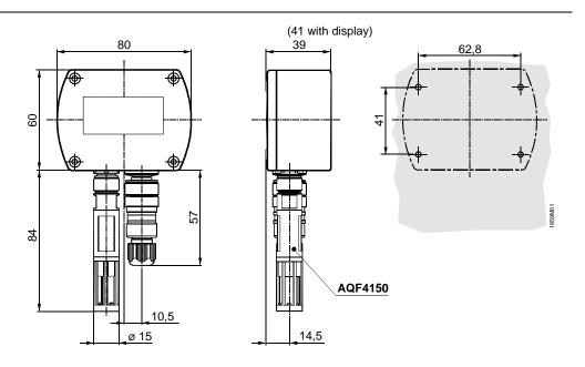
Dimensioning without (with) LCD-display
