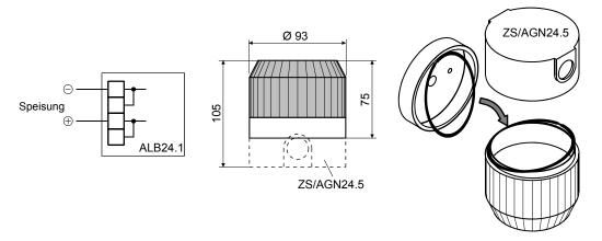
Remove rubber ring from the base and insert between housing and adapter base.
