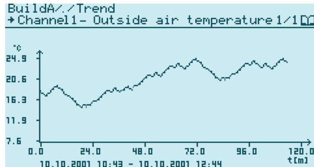
The PXM20 operator unit provides the user with five channels for trend logging, enabling 5 data points to be logged.
