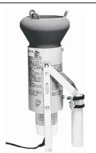
• This detector tester contains a hot air generator. For the performance check, the tester is pushed over the detector. The hot air released heats the detector and so actuates an alarm.
