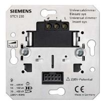
The universal dimmer insert sys 5TC1 230 is a flushmounted device for switching and dimming various electrical loads. Incandescent lamps, high voltage halogen lamps and low voltage halogen lamps with intermediate conventional or electronic transformers can be controlled.
