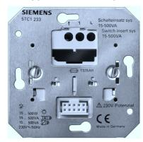
The switch insert sys 5TC1 233 is a flush-mounted device for switching various electrical loads. It is possible to control incandescent lamps, high-voltage halogen lamps and low-voltage halogen lamps with seriesconnected, conventional or electronic transformers.
