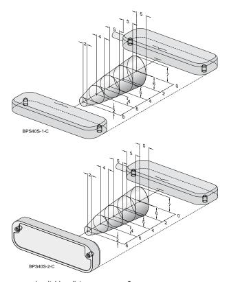
assured switching distance:  $s_{ao} = 8 \text{ mm}$ assured switch-off distance:  $s_{ar} = 18 \text{ mm}$
