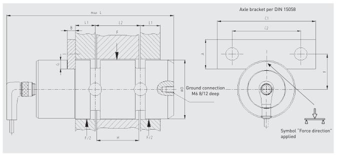
Dimensions: The customer-specific load pin drawing for the specific article number applies above all. For the F5301/F53C1/F53S1 series, there are no standard dimensions. All dimensions in mm.
