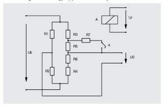
tecsis force transducers are working with four variable resistors (R1...R4) connected to a Wheatstone Bridge. Caused by deformation of the body the respective opposite resistors are lengthened or compressed in the same way. This results in an unbalanced bridge and a diagonal voltage U0.
