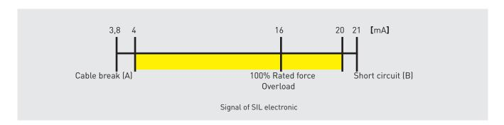
With a fixed signal level of, for example, 4 mA, the testing cycle can be triggered in every operating status upon activation of
