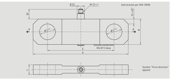
Dimensions: The customer-specific transducer drawing for the specific article number applies above all. For the F7301/F73C1/F73S1 series, there are no standard dimensions. All dimensions in mm.
