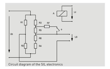
The switching of the resistor R7 causes a defined, always consistent, unbalancing voltage of the zero point (diagonal voltage) of the Wheatstone bridge. An external control unit, independent of the load cell (2-channel for safety reasons), can now activate relay A which changes the output signal of the force transducer by a defined value. If the expected change
