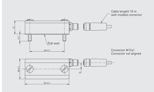
The strain transducer is to be affixed with a torque of 12 Nm on each screw (DIN EN ISO 4762 M6 x 16 – 10.9).
