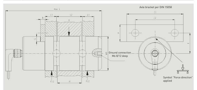
Dimensions: The customer-specific load pin drawing for the specific article number applies above all. For the F5308/F53C8/F53S8 series, there are no standard dimensions. All dimensions in mm.
