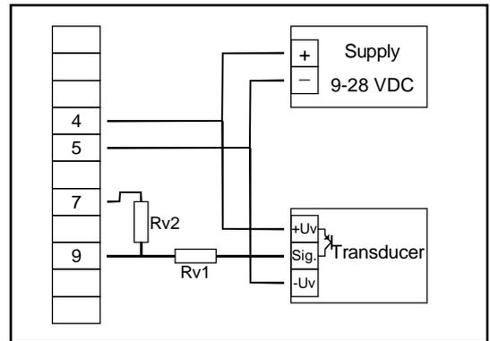
Connecting of a transducer (without individual power supply)
