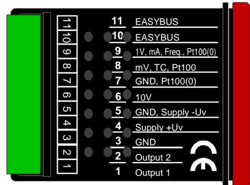
*Hint: The contacts 3, 5 and 7 are connected internally.*
