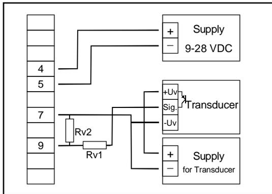
Connecting of a transducer (with individual power supply)
