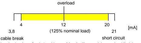
With activating the check relay a fixed signal jump of 8 mA will exceed the overload limit in every working condition. The measurement's upper limit of 20 mA however will never be reached. This makes the checking of the signal jump possible.
