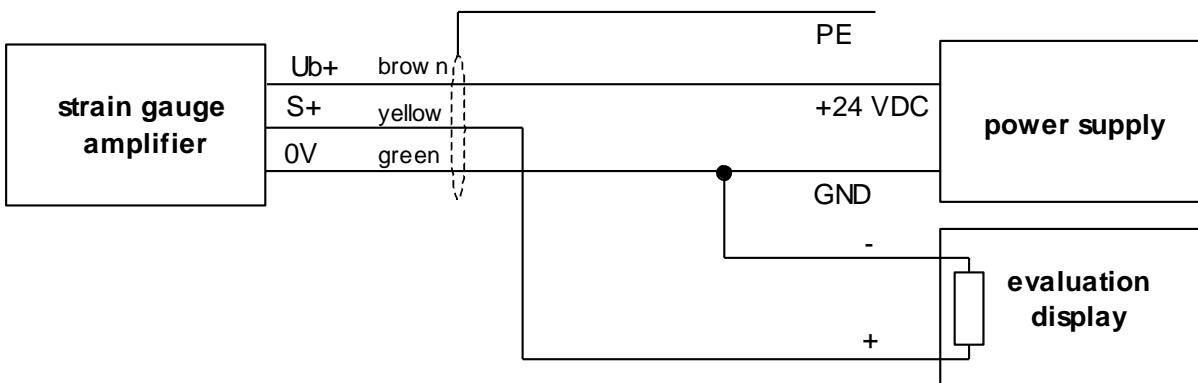
also for load cells with integrated amplifiers (0 (4) ... 20 mA, 0..10 V, 3-wire system)
