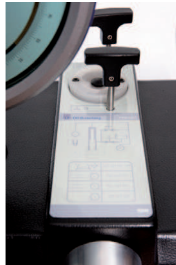
Control schematic on the CPB3800HP instrument base
