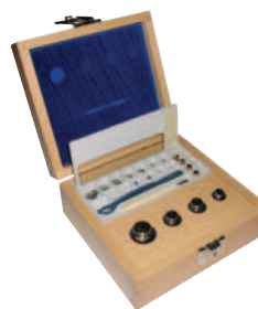
Set of fine increment masses
