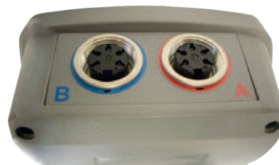
2 connection port for temperature probe inputs
