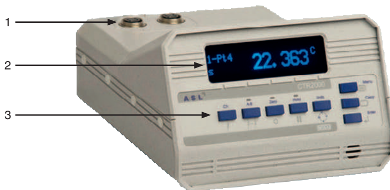
8-Channel precision thermometer, model CTR2000
