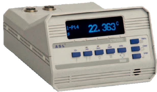
2-Channel precision thermometer, model CTR2000
