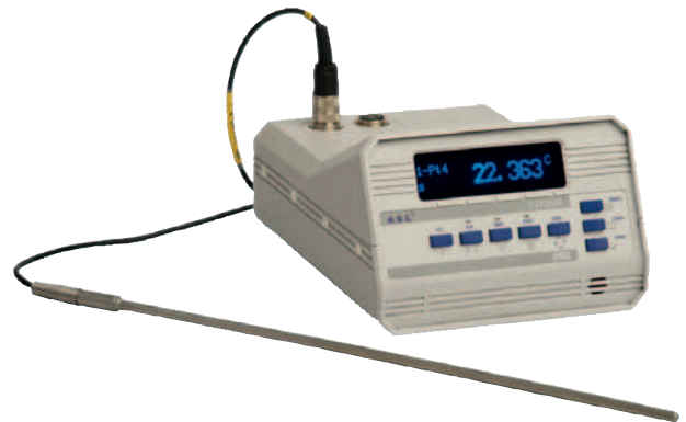
Precision thermometer, model CTR2000
