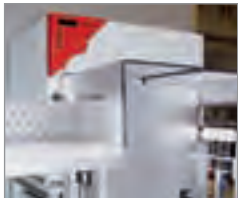
Integrated drying oven in a conveyor operation
