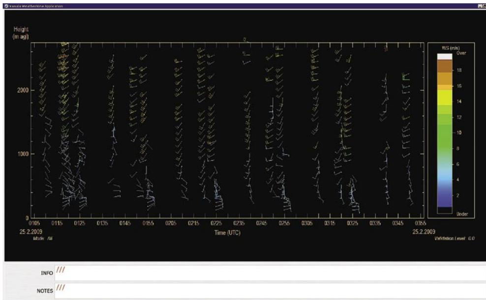
between these limits. Data can be shown in table format with wind data, wind shear warnings, or as a vertical profile of wind barbs for every layer measured on a separate row. Color-coding and audible alarms are used to easily identify the severity of the wind shear. The layers can overlap, totally or partially.
