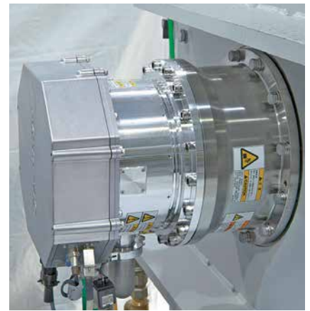
Energy saving turbomolecular pump
