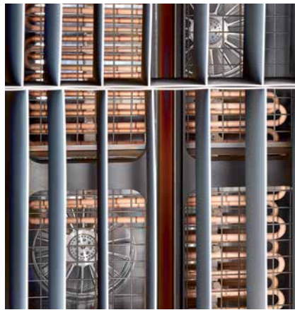
Turbomolecular pumps behind cold trap and chevron
