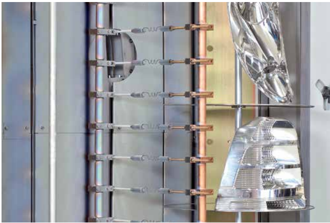
Evaporator and substrate inside the chamber
