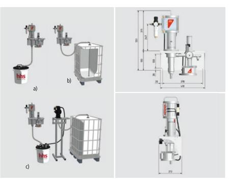
The compressed air driven piston pump delivers with upwards and downwards strokes and thereby creates an extremely consistent glue pressure. Due to quick regulation, the glue application remains constant even during changes in the production speed. The integrated pressure monitor automatically initiates an alarm if the pressure deviates from the set value. A fine filter at the pump output traps the smallest foreign particles and protects the dispensing system.
