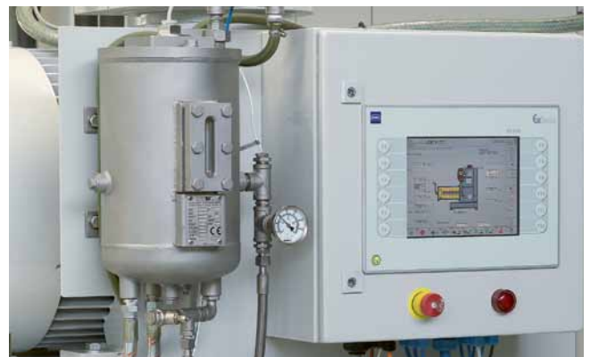
Control package PREMIUM: explosion-proof full version, fully graphic touchscreen panel with foil keys, emergency button
