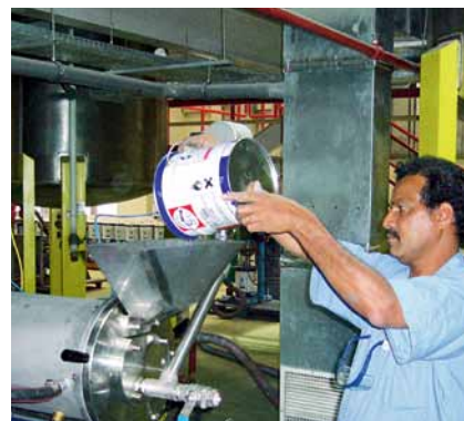
Preparation of a Cenomic™ with high-intensity cooling in a production plant for marine paint.
