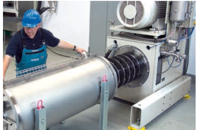
Fig. 5.2: Centex® T3 during removal of mill chamber – user-friendly handling of the large T series
