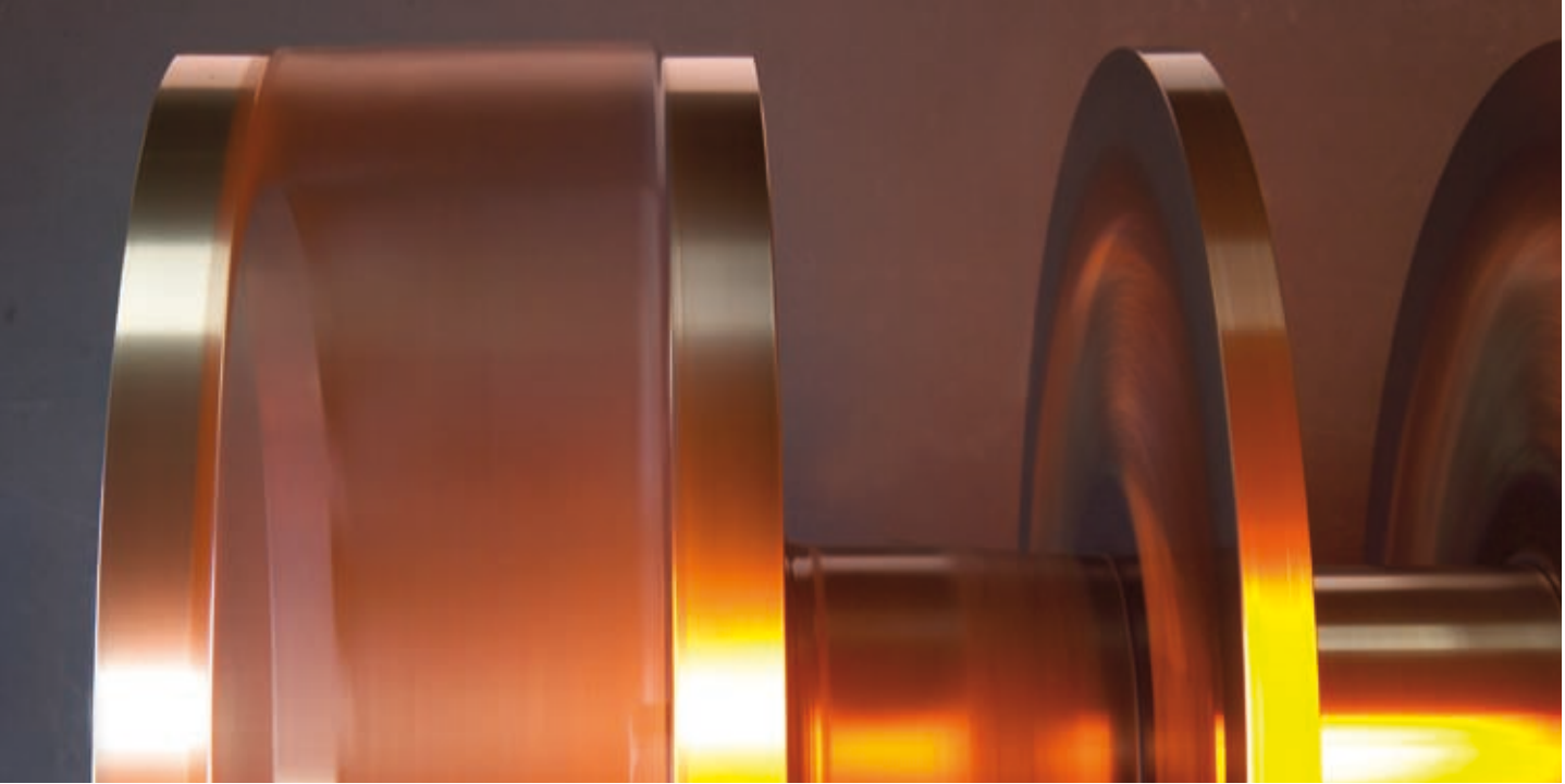
Fig. 4.1: Full-volume utilization by equidistant arrangement of grinding cells up to the deflector cage
