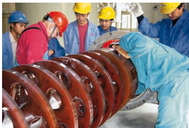
Fig. 6.3: Inspection of a metal-free Centex® T4 after one year of continuous operation in a milling plant for white pigments
