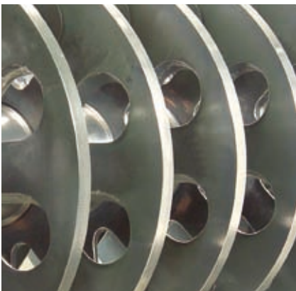
Fig. 5.3: Exchangeable counter flow conveying EcoMizer® discs from DraisResist® 84 in a Centex® T3
