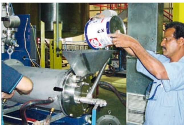
Fig. 6.2: Preparation of a Centex® L3 with high-intensity cooling in a production plant for marine paint
