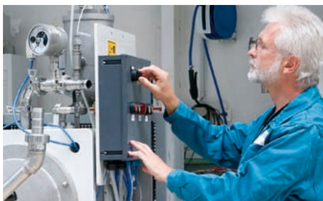
Fig. 7.1: Control package COMFORT: start/stop mill and pump, quicker/slower rotor, display speed/power, emergency button
