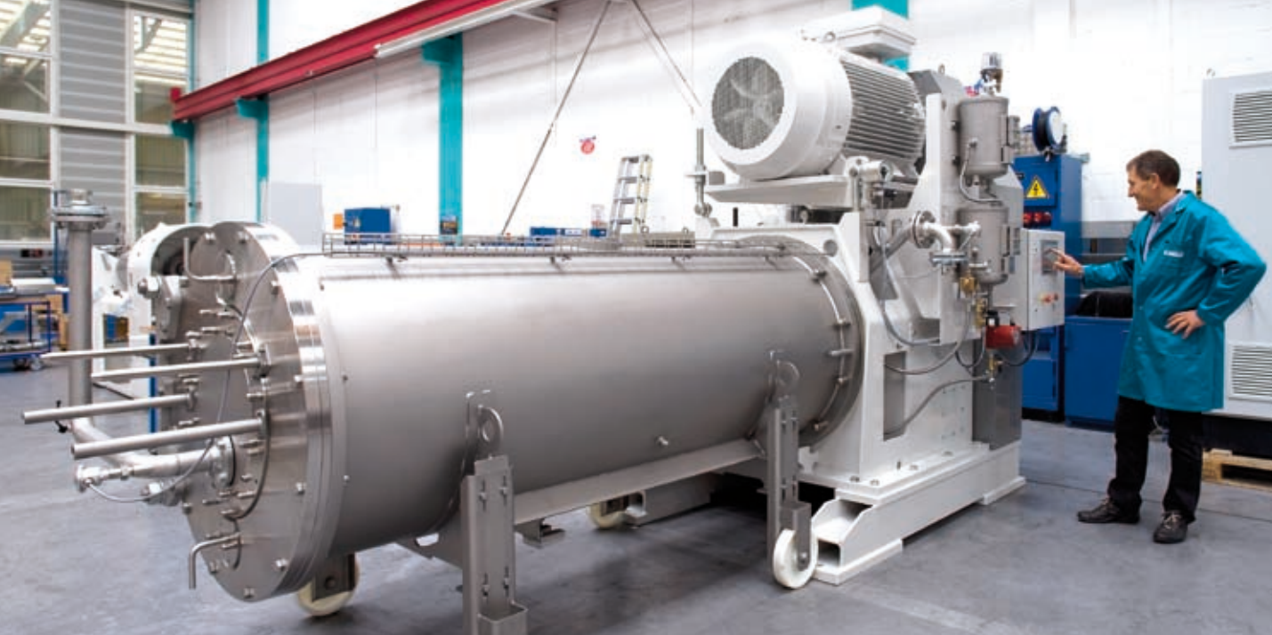
Fig. 6.1: Centex® T5 large Perl Mill® (drive power P = 355 \text{ kW} ) for the economical micro wet grinding of bulk material
