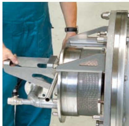
Fig. 5.4: Easy removal of a SuperScreen from a Centex® T3
