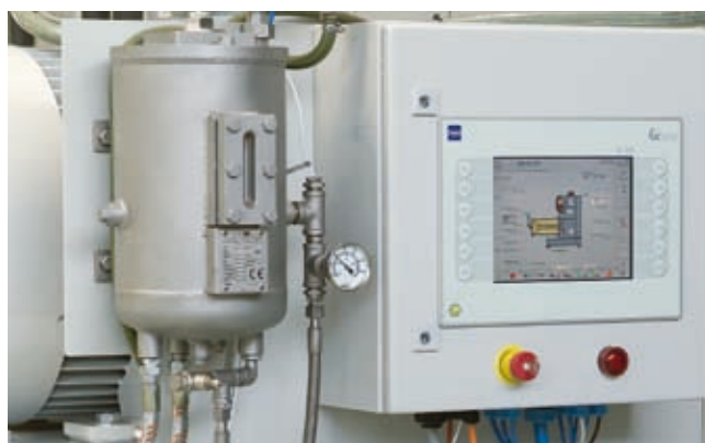
Fig. 7.2: Control package PREMIUM: explosion-proof full version, fully graphic touchscreen panel with foil keys, emergency button
