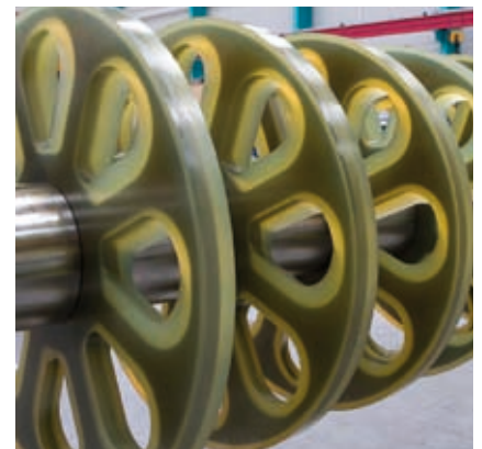
Fig. 5.5: Exchangeable counter flow conveying EcoMizer® discs from DraisElast® in a Centex® T5
