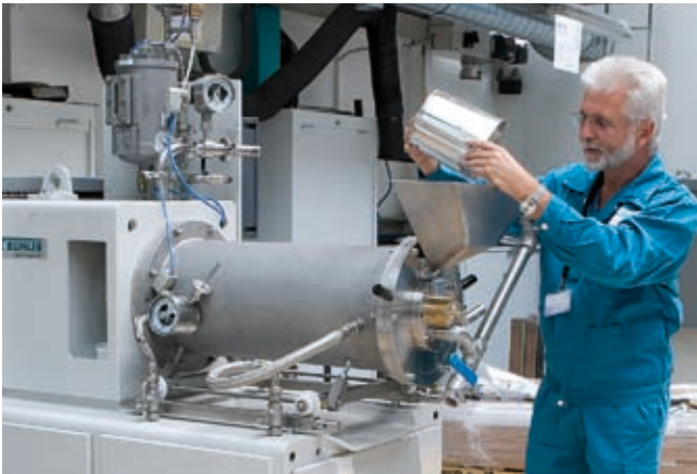
Fig. 5.1: Centex® L3 with outstanding functionality: filling of grinding beads through firmly screwed front-end speciality funnel
