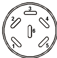
Figure 12: DIN socket for option analog output
