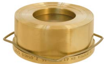
RK 41 with spiral centering PN 6 to PN 16, body material special brass, valve disc of austenitic steel
