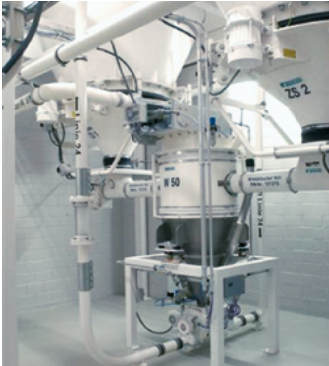
Conveying system equipped with high-grade components for materials discharge and feed, weighing and pneumatic conveying with airlock feeder.
