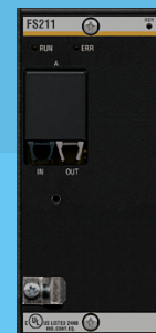
RMFS211 (.N) FAST-Bus Slave LWL 1x max. 150m (power pack 17W)
