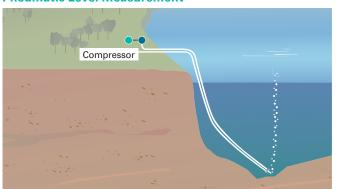
Sensor measures counter pressure produced by an air compressor and has no direct contact with water.
