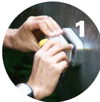
Clamp-on sensor on the pipe
