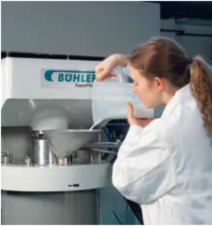
Fig. 9.1: Optimisation of grinding media filling degree of a SuperFlow® VCR 200
