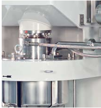
Fig. 9.2: SuperFlow® VCR 200 – grinding vessel lowered and pivoted
