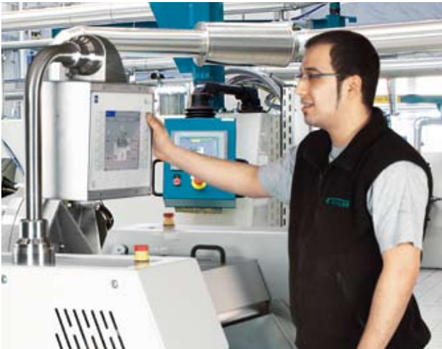
Fig. 4.1: PREMIUM control package with graphic touch screen panel
