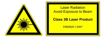
Z-Laser declares the conformity to a laser safety class according to EN ISO 60825-1 only for the complete product entity (fiber laser module and barreled optics module). Whenever this entity is changed the laser safety class is voided.
