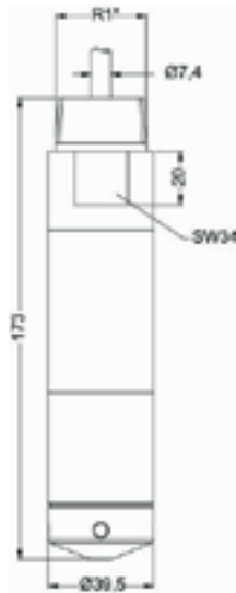
thread R1" for stainless steel pipe
