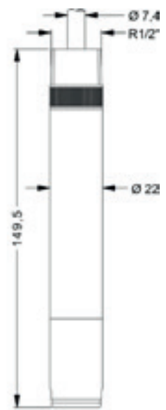
with thread R1/2" for mounting with stainless steel tube
