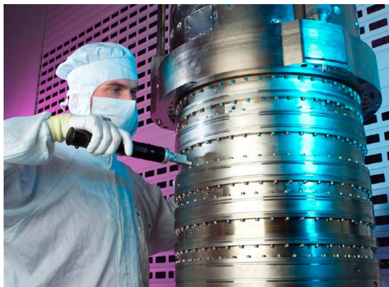
Capacitive displacement sensors are used for adjustment with nanometre precision of lenses in optical systems for wafer exposure.
