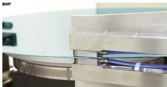
Wafer thickness measurement with two capacitive sensors
