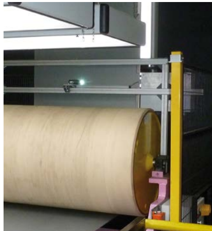
Measurement of the zinc sheet colour.
