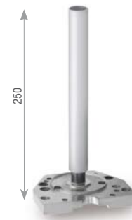
EDS/GPS-180-ZA-I(02) Eddy current long-stroke sensors with integrated electronics ▪ Measuring the piston position in the glass production ▪ Measuring range 180mm ▪ High shock- and vibration-resistance
