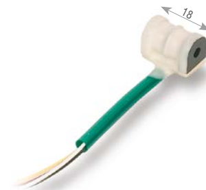
DTA-1D-20-DDV.02 LVDT displacement sensor with coated coil ▪ Measurement of a hydraulic valve position ▪ External electronics ▪ Measuring range 2mm ▪ Dipped paint seal
