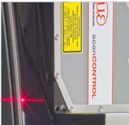
Gap measurement on a car body
