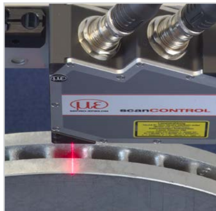
Profile measurements on brake disks
