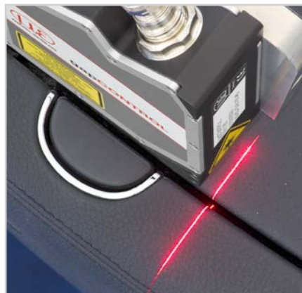
Distance measurement at the centre console
