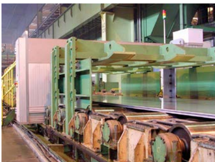
Thickness measurement in an aluminium hot rolling mill
