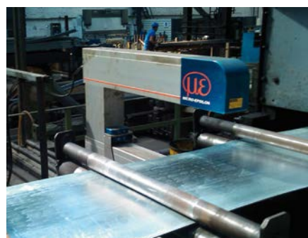
Thickness measurement in a forming line
