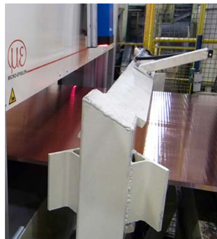
Thickness measurement in a milling line
