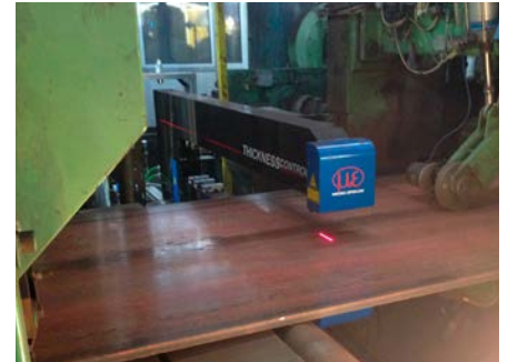
Thickness measurement in a milling line
