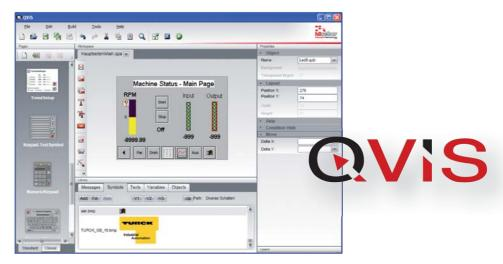
QVIS is the software environment used for visualization in the VT250 series. QVIS and CODESYS are closely linked to ensure an easy import of symbols for data exchange.
