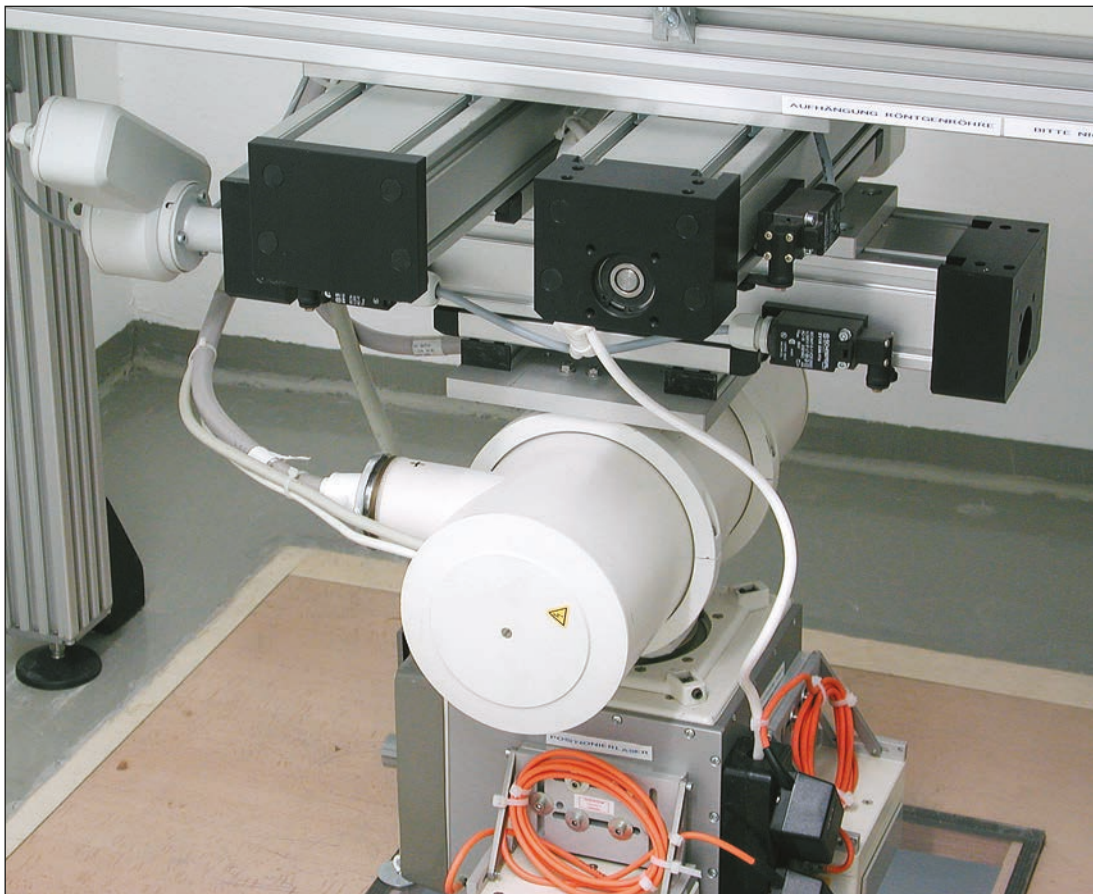
Suspension of an x-ray tube. X-Y adjustment of RK DuoLine S via EHL
