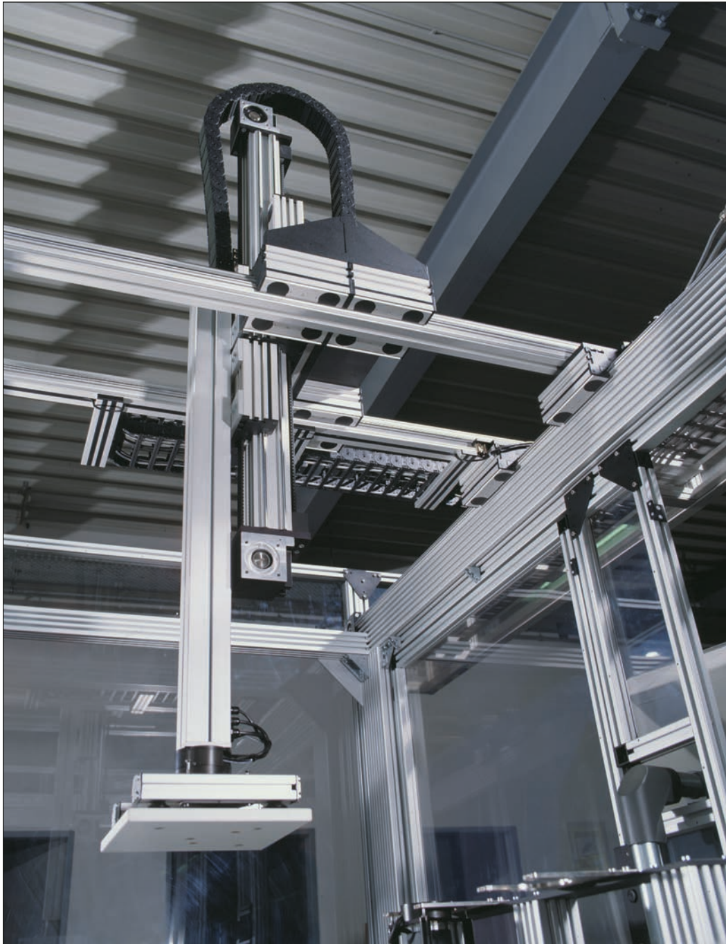
3-axis portal system of a machining centre
