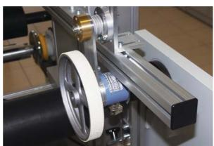
The industrially rugged WDG 58B encoder, in conjunction with the Wachendorff spring lever and a measuring wheel that has been mounted directly onto the encoder shaft, offers a easy method of accurate length measurement. To display the measured length or speed, simply connect a Wachendorff PAXI indicator, which can also provide the sensor power for the encoder.
