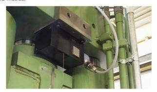
With these systems linear movement is detected by the unwinding of a steel wire from a precision drum. High precision mechanics ensure that the stainless-steel wire remains under constant tension and is accurately guided. Excellent linearity is thus obtained over the whole measuring range. The incremental or absolute encoder that is mounted onto the draw-wire system supplies accurate position data for the evaluation electronics.
