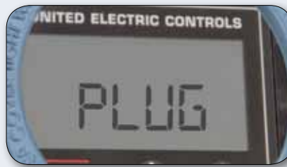
Diagnostics example: detecting plugged port
