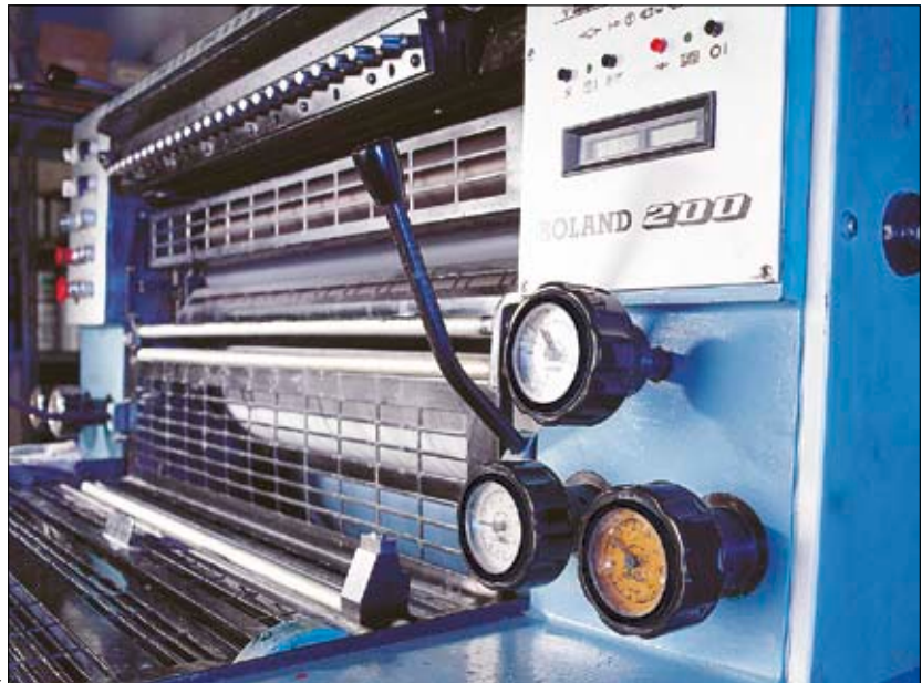
[1] Fine height adjustment of the saw blade of a circular saw. [2] Laminate coating system: Space monitoring during the coating process. [3] Tasty beer requires constantly controlled conditions: Control of mixing ratios in a brewery. [4] Control of roller pressure and ink mixing on small printing machines is still manual work. [5] A robust handwheel design is an important advantage in the metal processing industry.
