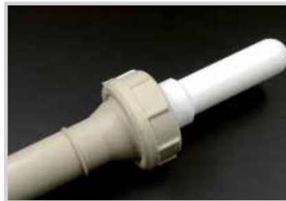
Plastic tube fitting system, suitable for type KAS-80-26-A-PTFE-PFS1-Y5. Tube length max. 2 m. With this fitting the user can install the sensor from the top and the sensor will reach up to 2 m deep into the tank.
