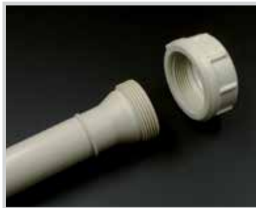
Plastic tube fitting system, suitable for type KAS-80-26-A-PTFE-PFS1-Y5. Tube length max. 2 m. With this fitting the user can install the sensor from the top and the sensor will reach up to 2 m deep into the tank.
